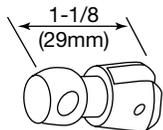
994M Swivel Armature (cannot be used with extension spacers)
